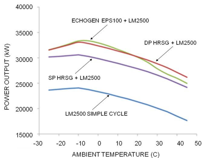
**Figure 4:** Performance model comparison between a standalone LM2500 gas turbine versus LM2500 combined cycle systems based on Echogen, single- and double-pressure steam and ORC technologies.
