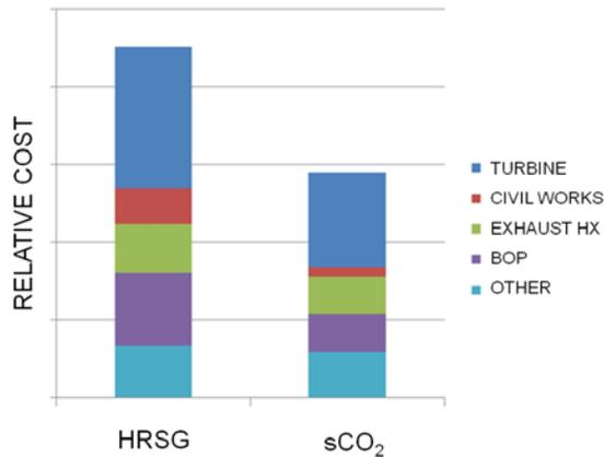
**Figure 5:** Compared to HRSG, an Echogen heat engine is estimated to cost less by 40 percent due to a more compact equipment set, smaller system footprint and lower balance of plant requirements for supercritical CO<sub>2</sub>.
