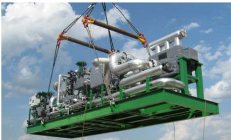
**Figure 2:** The first production unit of the EPS100 7.5 MWe heat engine is completing factory checkout tests at Dresser-Rand.
