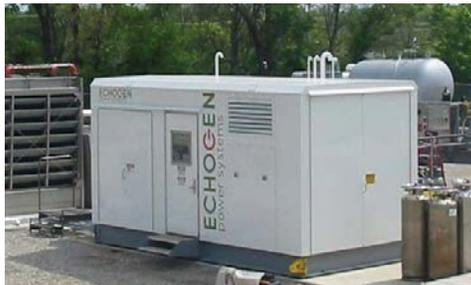
**Figure 3:** The EPS5 300 kWe, heat engine is derived from the 250 kWe demonstration system (above) which has completed checkout testing and is now in endurance testing.
