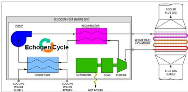
**Figure 1:** The supercritical CO<sub>2</sub> power cycle.
