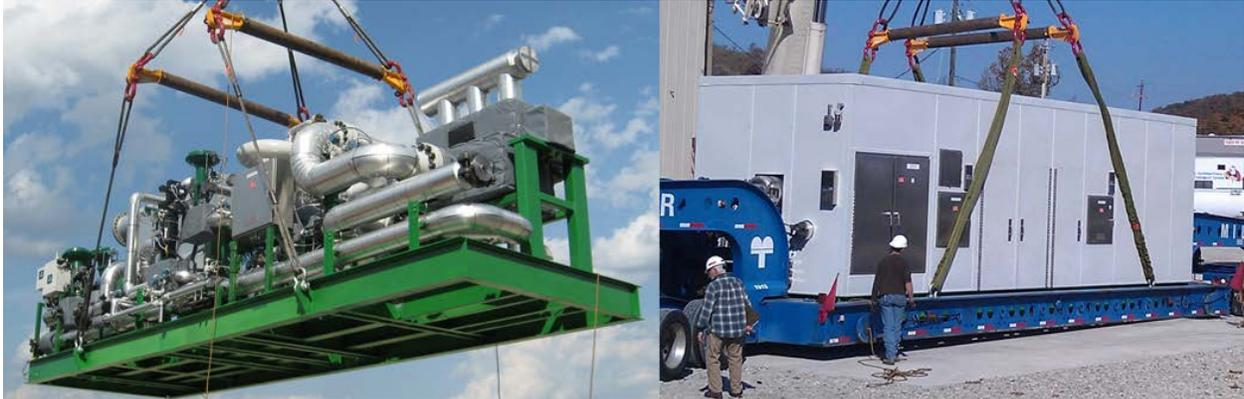
Figure 2: EPS100 sCO<sub>2</sub> heat engine, process and power skids
